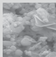
x50,000 SEM Octacalcium phosphate crystal embedded on the surface
